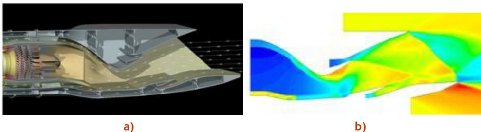
**Figure 3.** flows with shock waves in three-dimensional nozzle of ADVENT type (Bulat, Zasukhin & Prodan, 2012).
