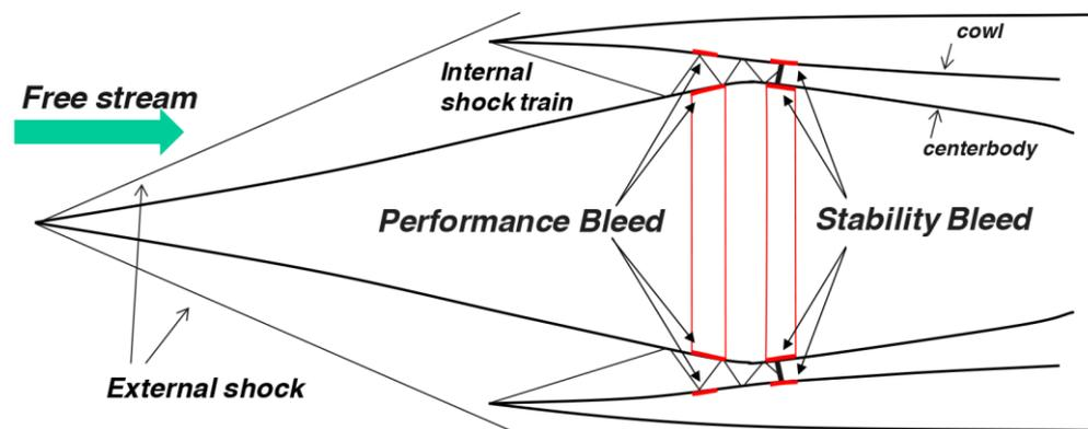
**Figure 2.** The air intake with a mixed (internal and external) compression
