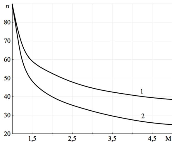
**Figure 8.** The angle  $\sigma$  of the first (1) and second (2) oblique shocks in optimum triple shock wave structure
