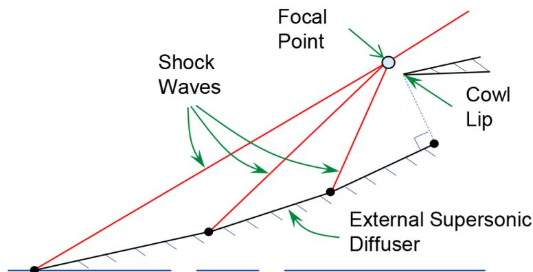
**Figure 1.** The air intake with external compression
