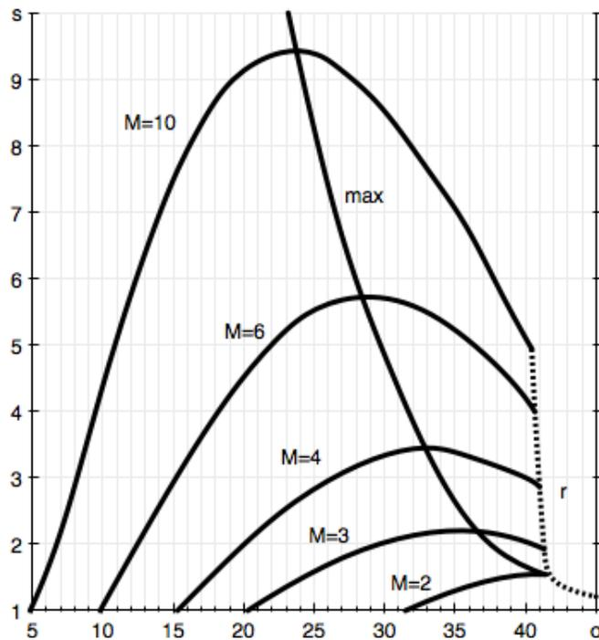
**Figure 9.** The dependence of the degree of increase in  $S$  stagnation pressure of the system fall-present, reflected and direct shock waves from the angle of the first shock and Mach number  $M$ .
