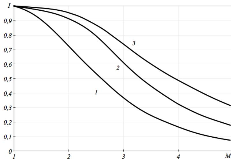
**Figure 7.** The total pressure recovery ratio behind the shock system.
