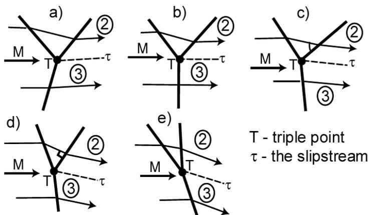
**Figure 6.** Triple configurations of shock waves. a) 1-TC, b) TC-1/2, c) TC-2, d) TC-2/3, e) TC-3, 2 - second shock (reflected for cases a-d, incoming for case e), 3 - the main shock
