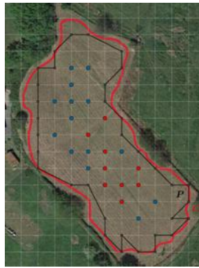
Figure 9. Lattice polygon P defined within the contour C (Source: Aerial orthophotography from SIGPAC (visorSigPac v4.8, https://sigpac.mapa.gob.es/fega/visor ), Fondo Español de Garantía Agraria, Ministerio de Agricultura, Pesca y Alimentación, Gobierno de España, licensed under CC BY 4.0; annotations by the authors)
