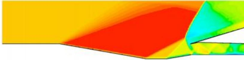
**Figure 4.** Flow around the air intake on non-isobaric mode
