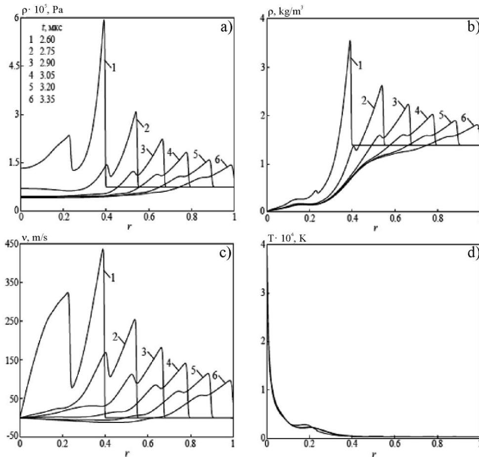
**Figure 3.** The distribution of pressure (a), density (b), velocity (c) and temperature (d) in the aureole vapour of the particle
