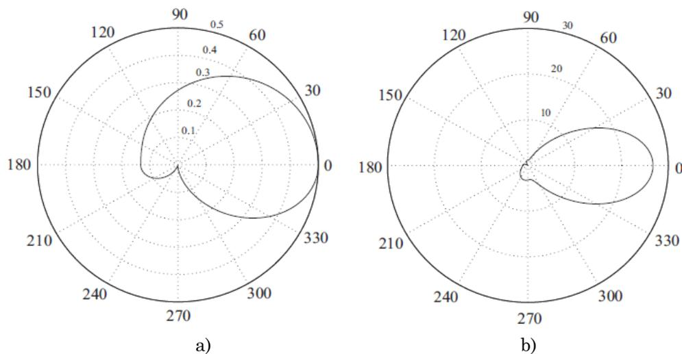
**Figure 2.** Distributions of radiation intensity when  $x=1$  (a) and  $x=2$  (b)
