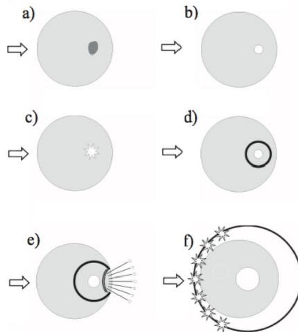
**Figure 1.** Development of interaction process of laser radiation with a droplet: a) radiation focusing; b) the formation of vapour bubble; c) the formation of plasma cloud; g) the emergence of a shock wave as a result of the explosion of plasma formation; d) the arrival of a shock wave to the droplet border, ionization of gas surrounding the droplet, ejection of small droplets into the environment; f) the occurrence of free electrons flow
