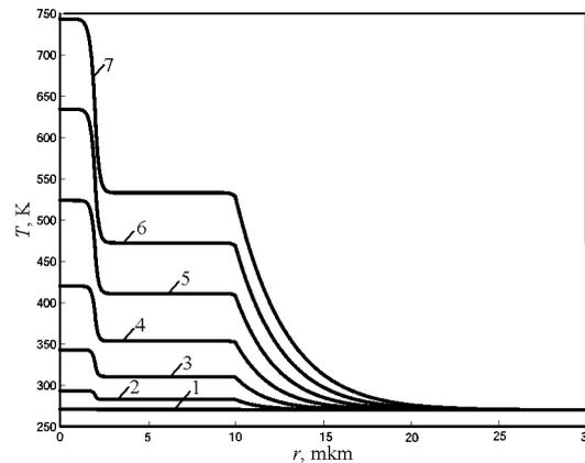
**Figure 2.** Temperature field around the water droplet at  $Q=20$  J
