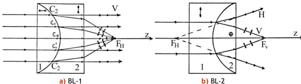
Figure 1. Two types of bifocal lenses
