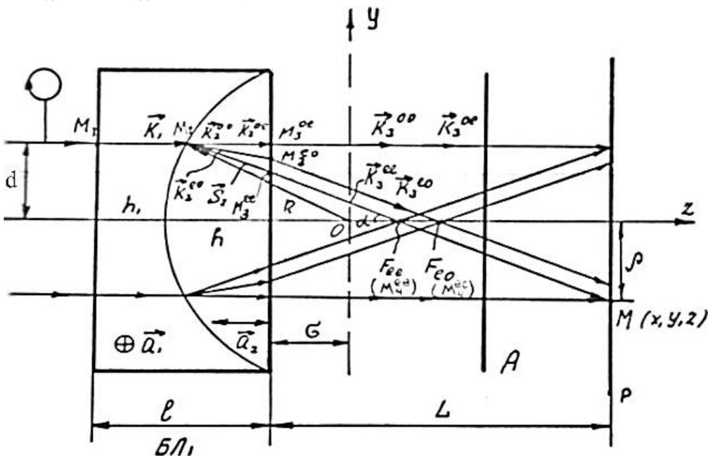
Figure 3. Electromagnetic wave propagation through a bifocal lens of BL-1 type
