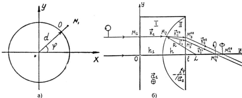
**Figure 2.** Propagation of electromagnetic waves through the anisotropic crystalline lens made of  $\text{CaCO}_3$  uniaxial crystal.
